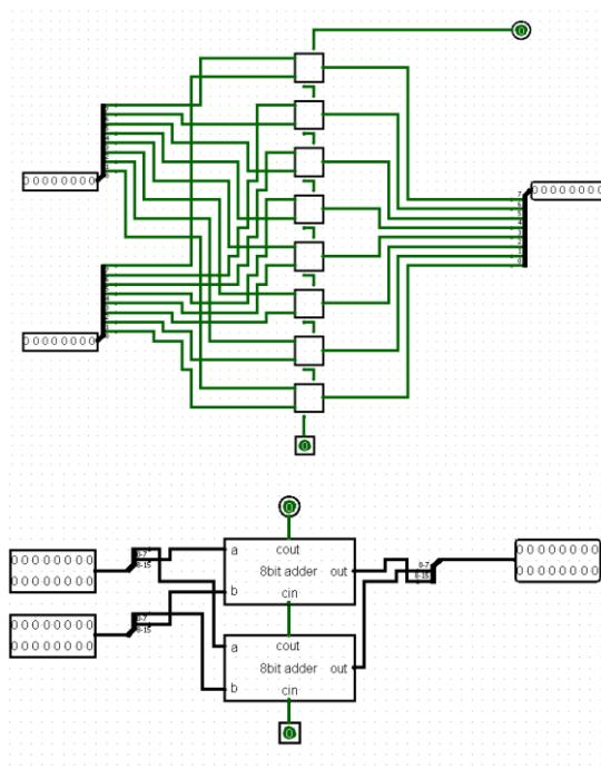
I started by developing the ALU of the CPU, not knowing much about the control aspect initially. I created a full adder and then instantly created an 8-bit adder by chaining 8 of them together. However, I did not consider the placement of pins and wiring very well, so it turned out to look a bit convoluted (but still functional). I further fumbled pin placement when I made a 16-bit adder for the a 16-bit PC, which led to very interesting connections to splitters.
